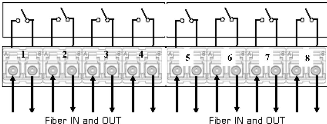
Note that the 1x1 switch is between each LC port. You can have as many 8 pair of fiber cables connected through this device to simulate fiber-cut fault scenario.
