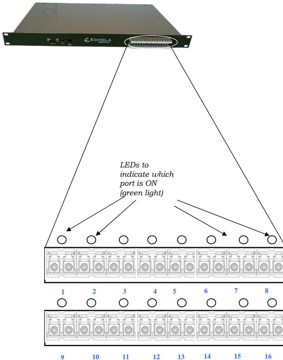
Each LC connector has two input/outputs marked as B and A (duplex). Suppose if you want to simulate fiber cut scenario between 2 optical devices.
