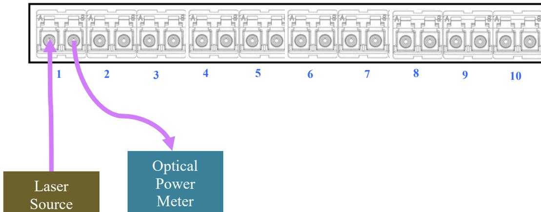
Each port has to be calibrated individually. Although the above diagram shows the setup for one port, you will have to repeat the same calibration procedure for all ten ports. The laser source can be either 1310nm or a 1510nm wavelength or a tunable laser depending on production requirement.
