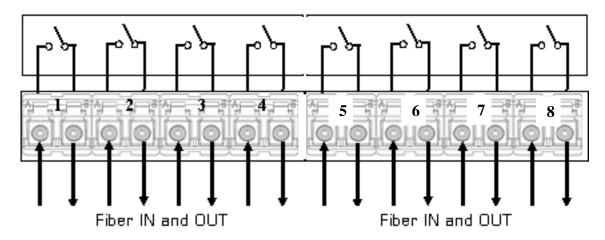
Note that the 1x1 switch is between each LC port. You can have as many 8 pair of fiber cables connected through this device to simulate fiber-cut fault scenario.
