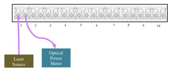
Each port has to be calibrated individually. Although the above diagram shows the setup for one port, you will have to repeat the same calibration procedure for all ten ports. The laser source can be either 1310nm or a 1510nm wavelength or a tunable laser depending on production requirement.
